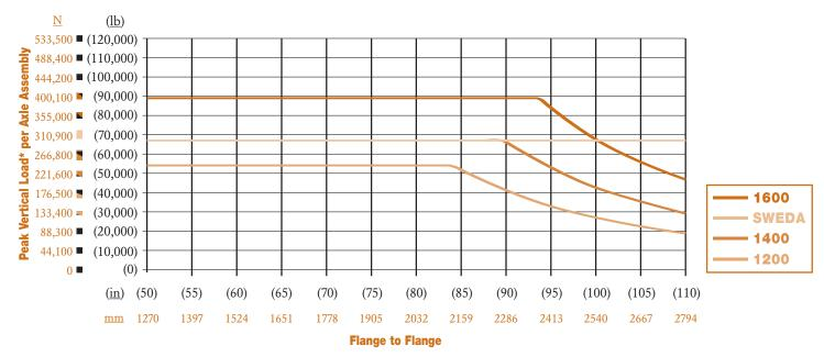
\*Peak load level (fixed axle) assuming traction-limited condition, 0.5 traction coefficient, and a specified loaded tire rolling radius.
